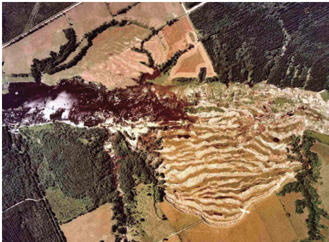
Fig. 2. Typical retrogressive landslide in sensitive clay: the South Nation River slide of 1971 (© 2008, produced under license from Her Majesty the Queen in Right of Canada, with permission of Natural Resources Canada, courtesy of the National Air Photo Library).
