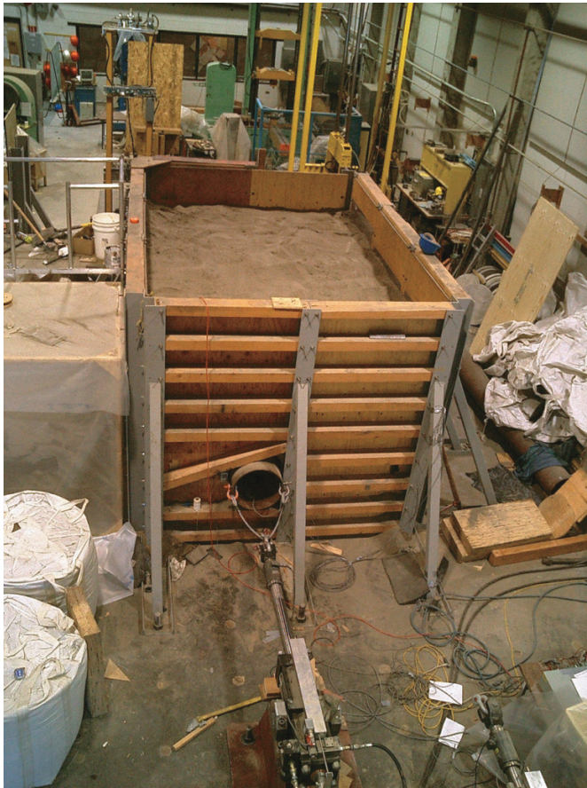
Fig. 1. Test configuration showing the soil chamber and hydraulic actuator set up for an axial pullout test.
