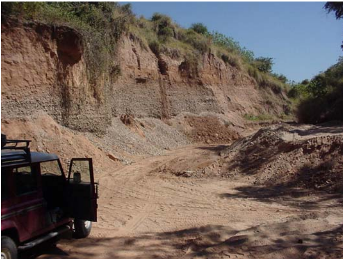
Figure 7. Wind blown sandy silt (loess) overlaying cobble gravel with sand lenses at a tributary valley near to the crossing.
